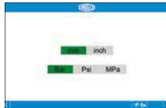
The currently set unit of measurement is displayed in green. Tapping a key sets the corresponding unit of measurement.
