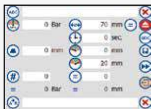
Easily input pressure, hold time, aperture diameter, pre-selection counter and crimping dies.
