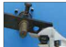
Blade adjustments for skiving depth need only to be made once for each hose dimension on the USM 10 S.
