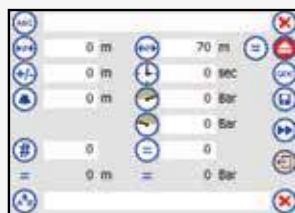
Easily input crimping dimensions, correction value, hold time, aperture diameter, pre-selection of counter and crimping dies (automatic).
