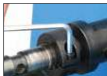
Easy adjustment of the skiving tool.
