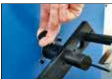
Easy exchange of skiving tool using a locking pin on USM 10 S.
