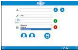
The RFID reader enables automatic logon to the machine with an RFID chip.
