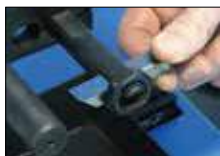
Skiving mandrels are manually adjustable.
